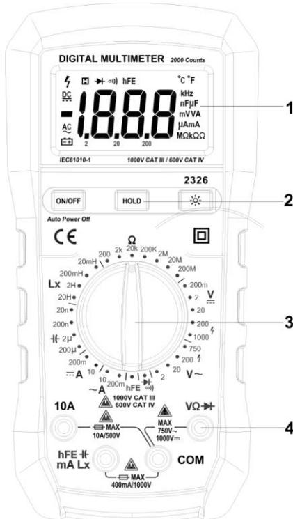
1 LCD display 2. Keypad 3. Rotary switch 4. Terminals
